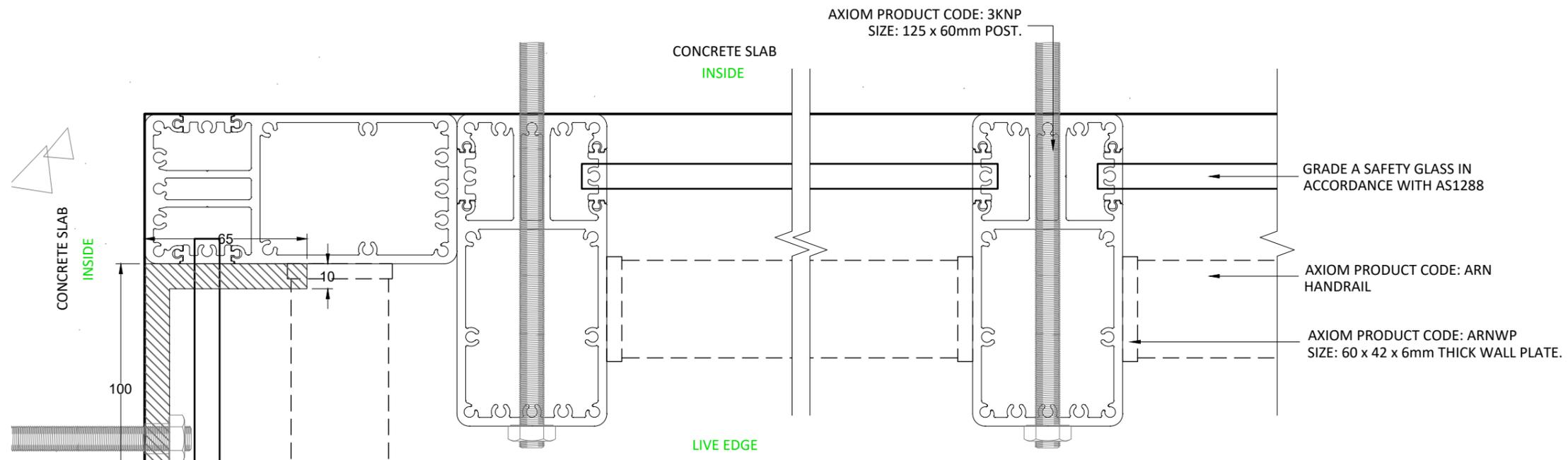
**PLAN VIEW - INTERNAL CORNER DETAIL**
