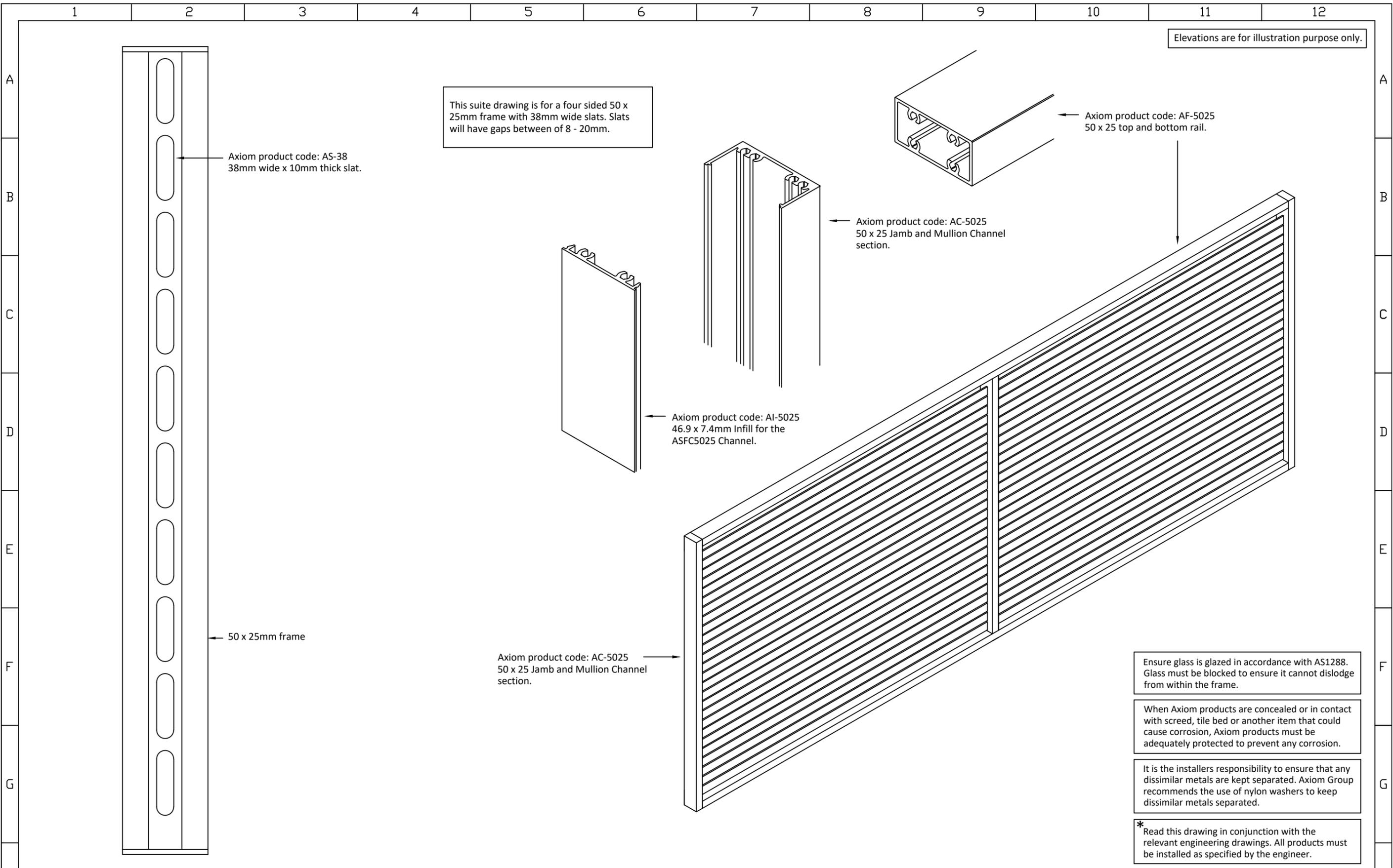
Ensure glass is glazed in accordance with AS1288. Glass must be blocked to ensure it cannot dislodge from within the frame.
