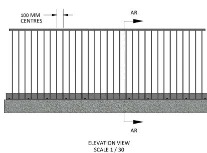
7. AXIOM ALFM FACE MOUNTED CHANNEL FIXED TO SLAB EDGE WITH 2N° M10 CHEMSET A4 / 316 STAINLESS STEEL ANCHORS VERTICALLY ABOVE EACH OTHER AND AT EACH END, THEN AT 300MM MAXIMUM CENTRES BETWEEN 90MM MIN. EMBEDMENT AND 50MM MIN. EDGE DISTANCE.
